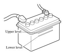
Inspect the electrolyte level at least once a week. If it's low, remove the caps and add enough distilled water to bring the level between the upper and lower level (illustration).
